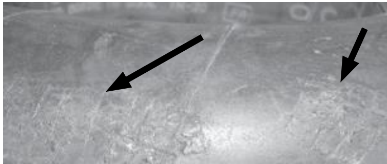
Sticker damage - damage of a tube from a tubeless tire without the removal of the stickers
